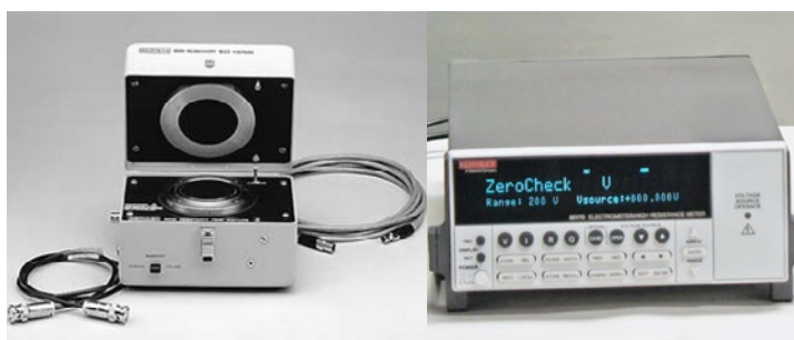
The EE 04TF volume resistivity test fixture combined with base instrument EE 01Base for determination of volume and surface resistivity on insulated materials.
