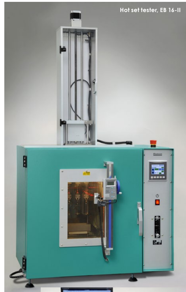
A computer, a digital calliper as well as clamps and weights for 8 samples are included with the EB 16-II.
