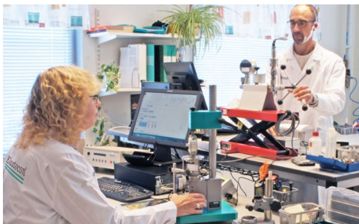
The general laboratory for calibration at 23 °C. In addition to this we have a constant room for calibration of length at 20 °C ± 0,5 °C, and a room for temperature calibration.
